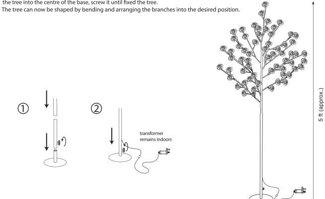
This product is suitable for indoor and outdoor use but please ensure the transformer remains **INDOORS** at all times. Always unplug from the mains supply whilst installing or maintaining.
